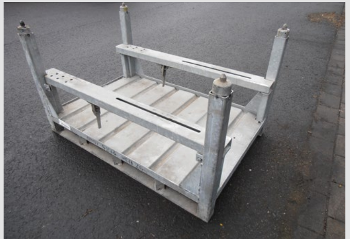
Steel frame for double-deck loading
