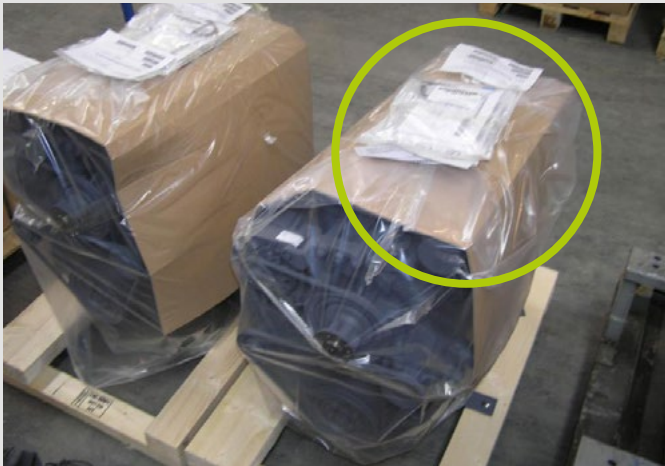
Accessories in bags fixed on the top of the engine = allowed
