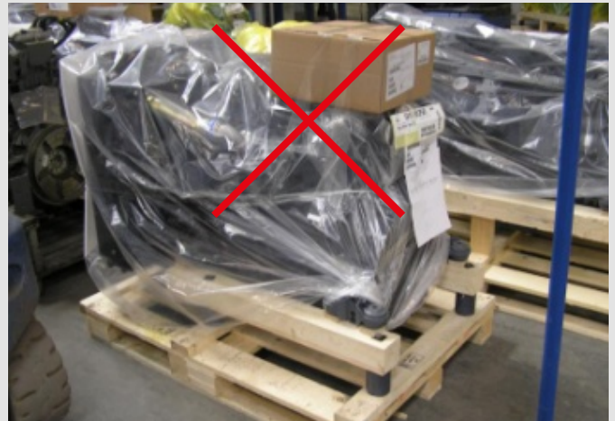
Accessories box fixed on the top of the engine = NOT allowed
