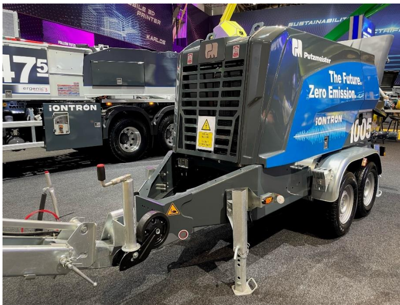
Caption: The PUTZMEISTER BSA 1005 iONTRON is powered by a 360-volt drive system from E-DEUTZ. Credit: DEUTZ AG
